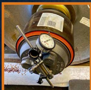
Check the bearing lateral with a dial indicator mounted on a magnetic base:
