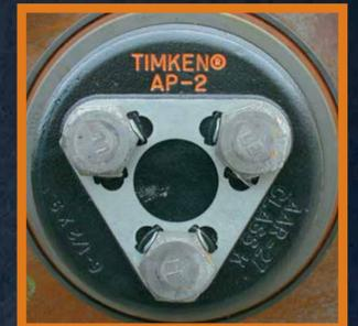
Lock the cap screws by bending all of the locking plate tabs flat against the sides of the cap screw heads.
